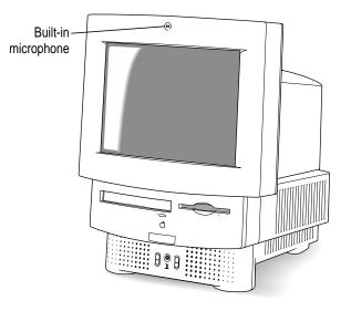
**WARNING** Do not stick any small objects into the built-in microphone. Doing so may damage your equipment.
